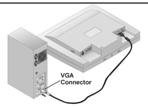
3. Make sure the signal cable is secure to both the monitor and PC. Tighten the connecting screws to ensure a secure connection.
